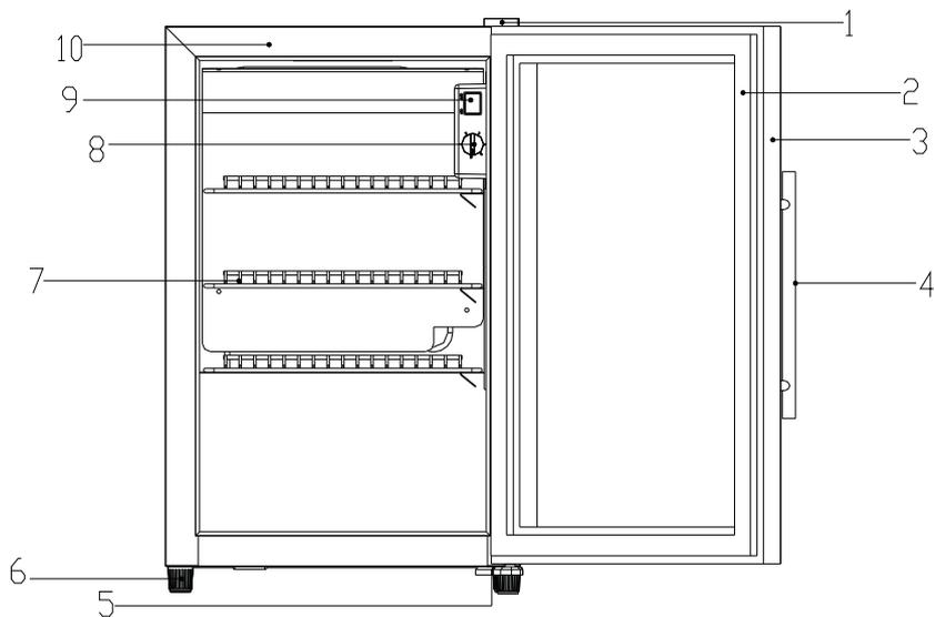
1. Hinge Cover 2. Door Gasket 3. Door Frame 4. Door Handle 5. Lower Hinge
